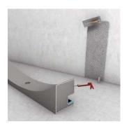
1 Apply a ½" bed of thinset mortar to the unit's contact area at the wall where the unit will be placed. Apply 4 continuous beads of wedi joint sealant to the bottom part (steel plate) in either direction. The bottom connects to the floor, when the unit is attached against the wall.
